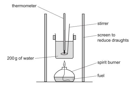
The initial temperature of the water and the temperature after heating by the fuel are recorded.
