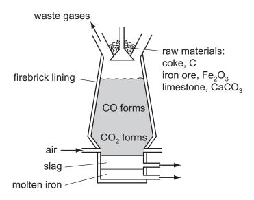
The coke reacts with the oxygen in the air to form carbon dioxide.
